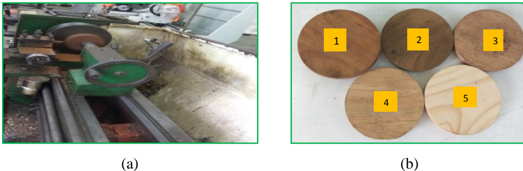
Figure 1 (a) Preparation of wood material by using CNC milling cutting machine (b) Wood materials (1) Pyinkado, (2) Teak, (3) Kanyin, (4) Rubber and (5) Pine
